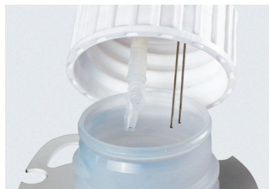
Sensitive level sensor to prevent liquid overflow
